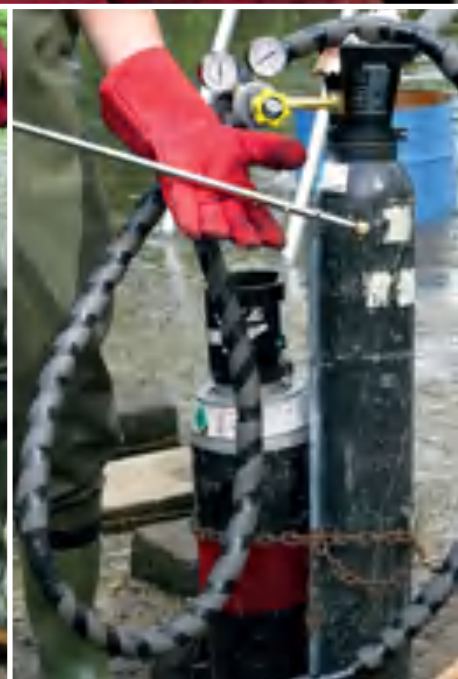
Figure 4.10 Carbon dioxide freeze corer (Photo John Davy-Bowker)
