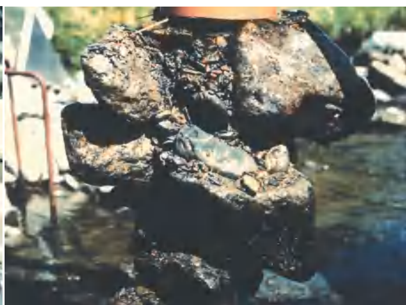
Figure 4.11 Material collected on a liquid nitrogen freeze corer (Photo John Davy-Bowker)
